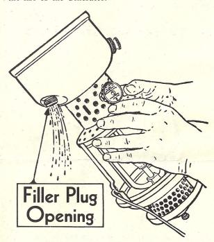
To drain, simply remove Filler Plug and pour gasoline out through Filler Plug opening. The Lantern will light more easily and better with fresh gasoline in the Fount. Whenever available, clean water-white undoped gasoline should be used; however, leaded gasoline and regular motor fuel can be used. CAU-TION: Always provide good ventilation—particularly when burning leaded gasoline.
